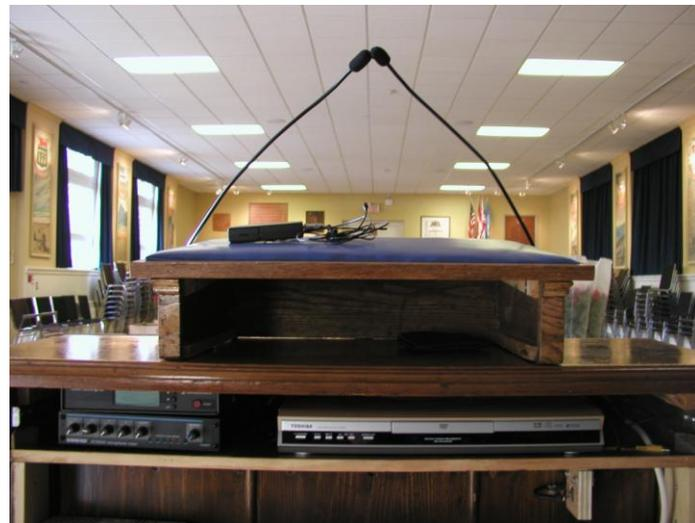
The two microphones in an X/Y configuration provide a very wide pick-up. The same mics are used for various stage productions
