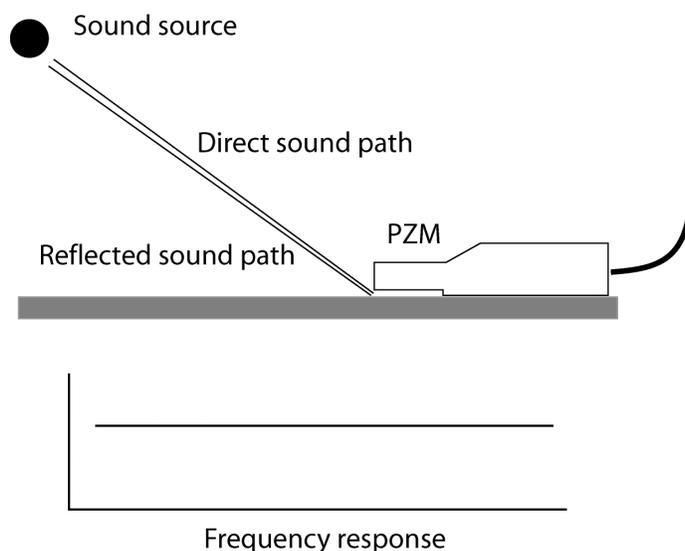
*Figure 7. In a boundary mic such as a PZM, direct and reflected waves add in phase at all frequencies in the audible band.*
