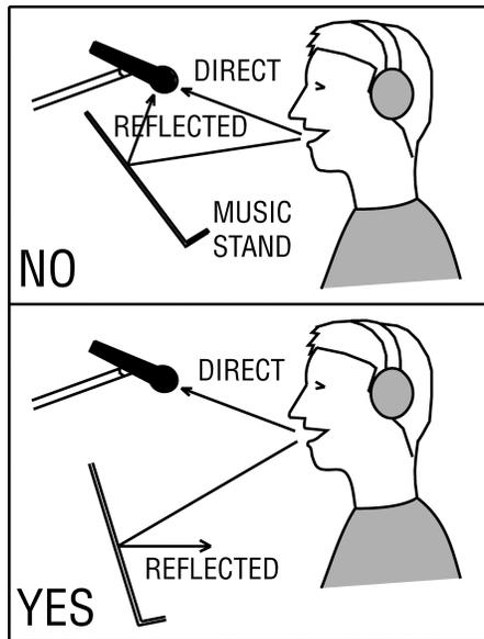
Figure 5. Top: Sound reflects off the music stand into the mic, causing acoustic comb filtering. Bottom: Sound reflects off the music stand away from the mic, preventing acoustic comb filtering.
