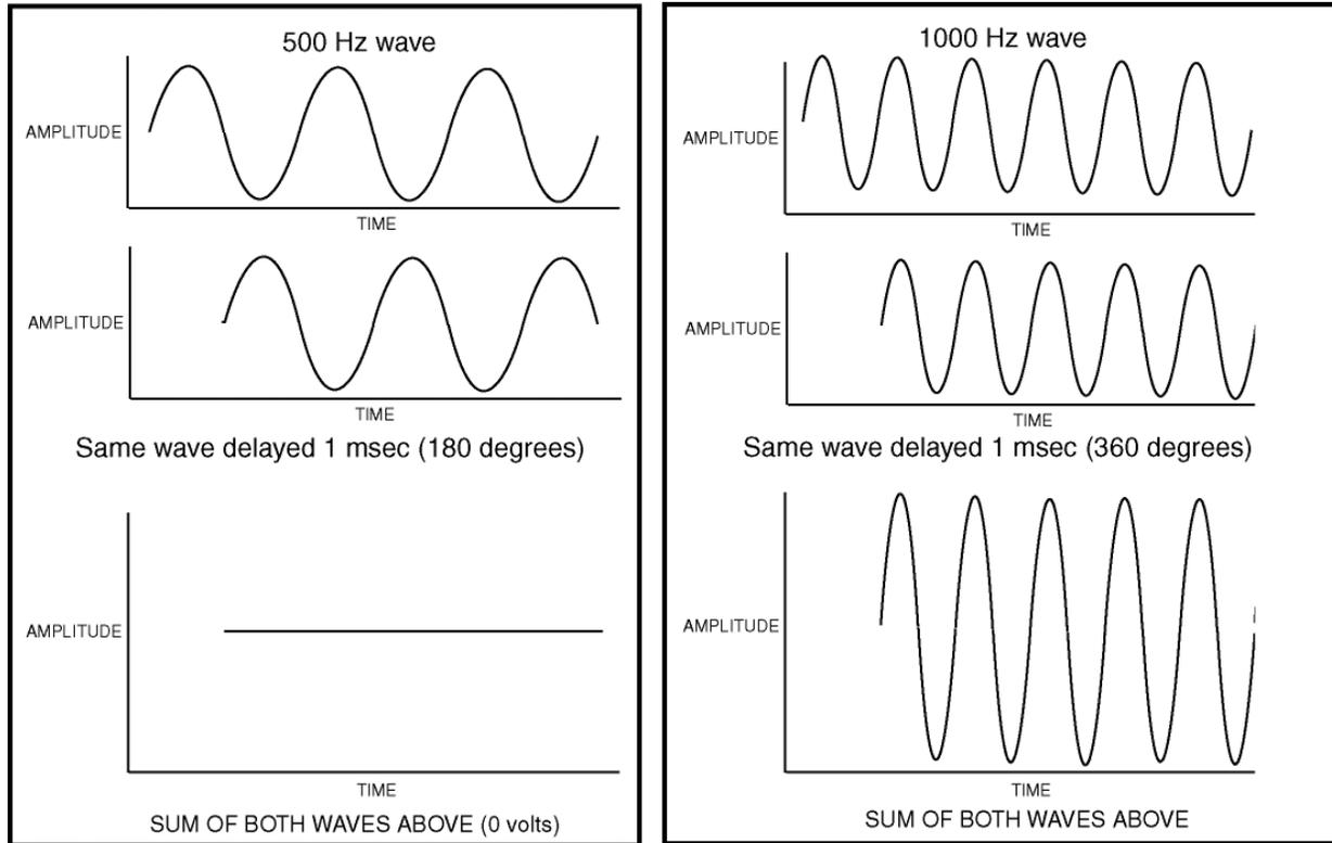
Figure 4. Two 500-Hz waves with a 1 msec delay in one wave cancel out when summed. Two 1000-Hz waves with a 1 msec delay in one wave add when summed.
