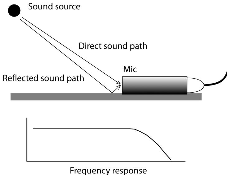
Figure 6. Direct and reflected waves cancel at high frequencies at the diaphragm center.
